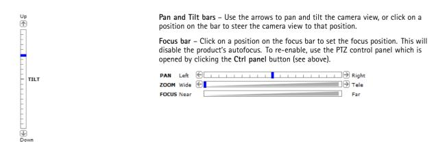
The PTZ controls can be disabled under PTZ > Advanced > Controls, see Controls on page 28.
